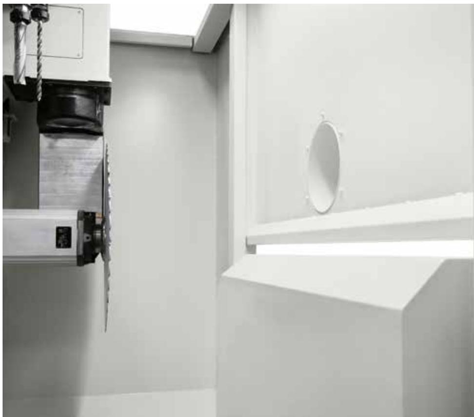
The extraction outlets are arranged around the perimeter of the cabin, in order to remove the the finest dust and keep the cutting area always clearly visible.
