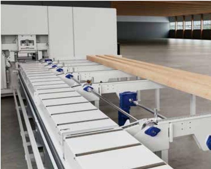
Consisting of a series of supports with variable spacing, it allows the loading of timber up to 16 metres long, 450 mm wide and 240 mm thick.
