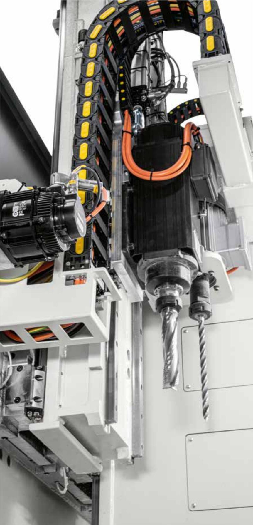
The 3-axis vertical drilling and routing units, compatible with drill bits and end mills, are dedicated to the execution of through or blind machining operations on the workpiece upper face.
