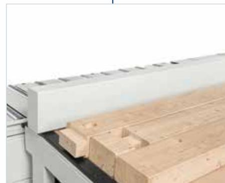
*Simple unloading of the processed element.* Easy storage and retrieval of elements, thanks to the parallel-branched unloading buffer.
