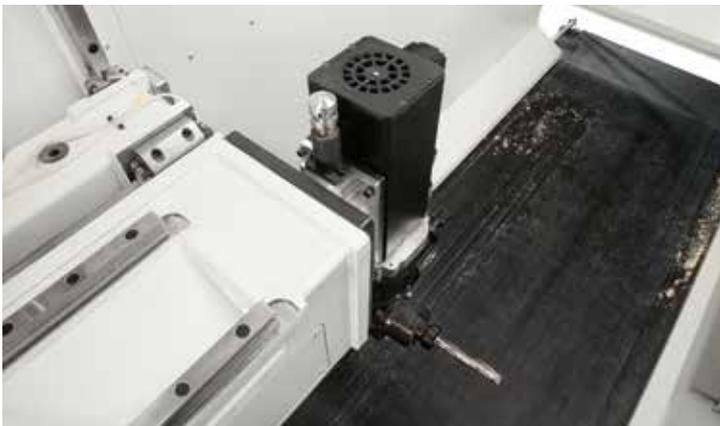
The pressurised ink pen is accommodated in a device that can take it out of the way when not in use.
