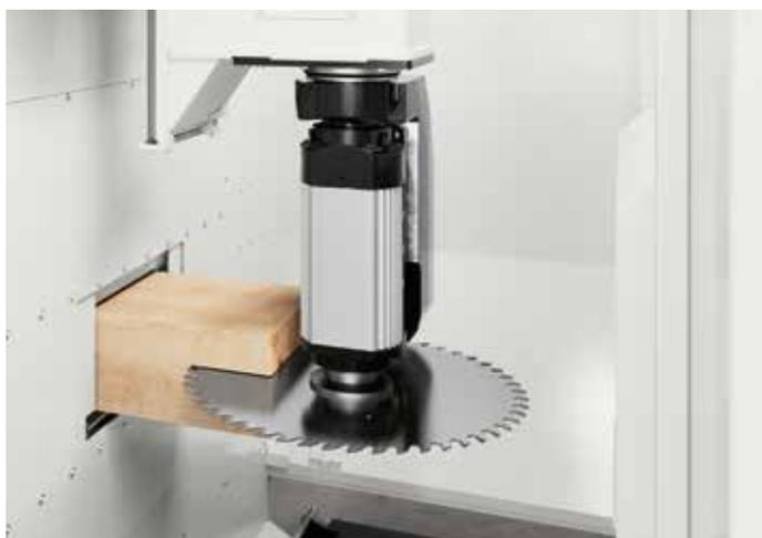
The most common operations that can be performed with the saw blade unit are straight and inclined cuts, slots for hardware, slopes and notches.
