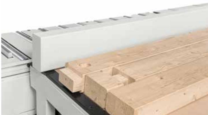
A mechanical pusher pushes the element onto the storage buffer, composed of fixed supports arranged at variable spacing. Their inclination and the presence of idle rollers allow rapid retrieval of the elements.
