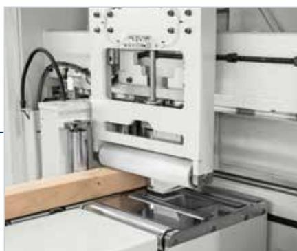
*High precision* ensured by horizontal and vertical pressure rollers that avoid vibrations of the workpiece during processing.
