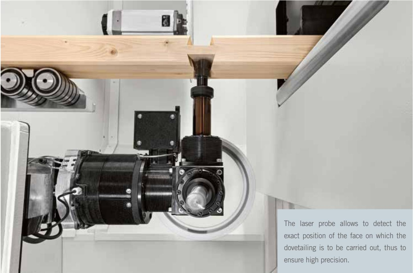
The laser probe allows to detect the exact position of the face on which the dovetailing is to be carried out, thus to ensure high precision.
