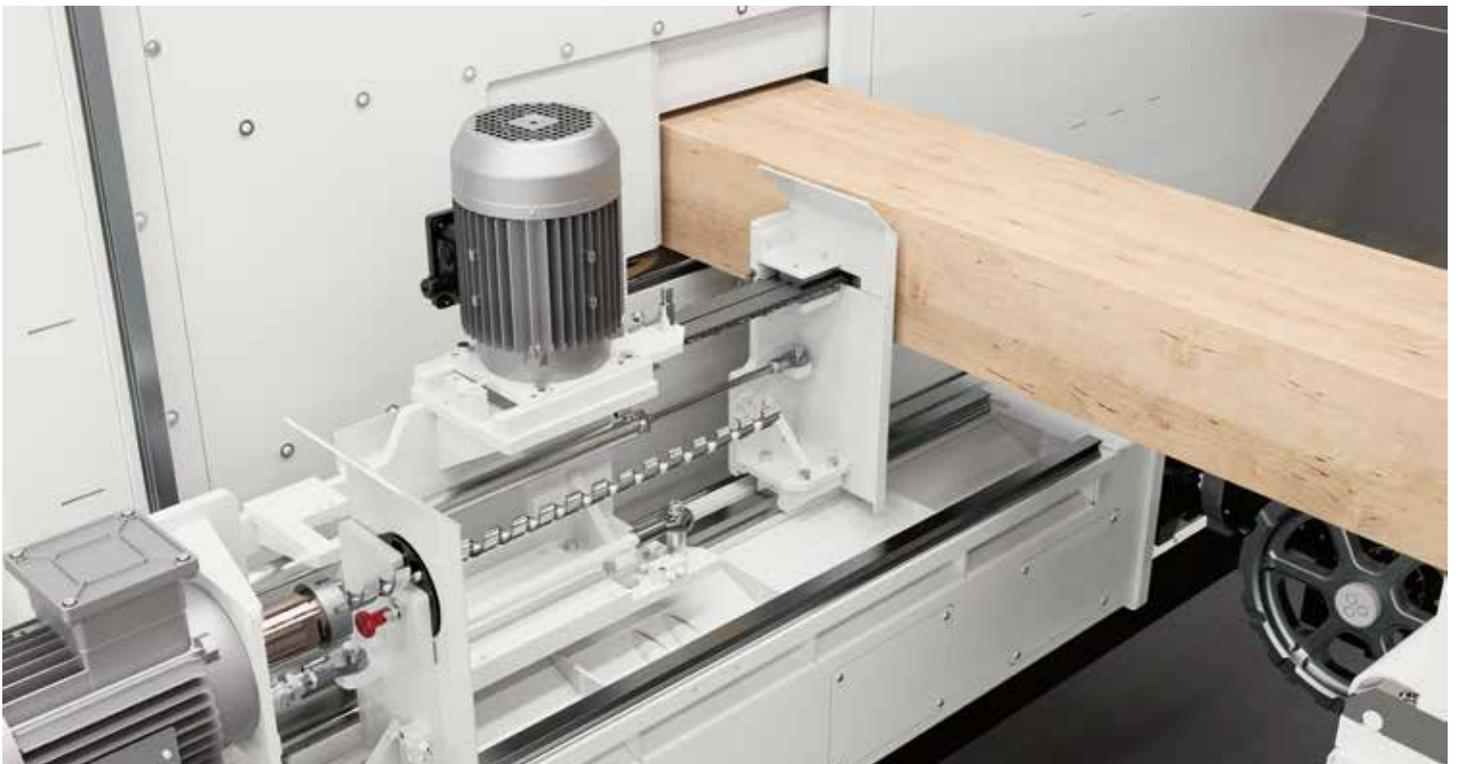
Thanks to the horizontal mortise chain unit, it is possible to execute through or blind hardware slots of up to 450 mm depth.
