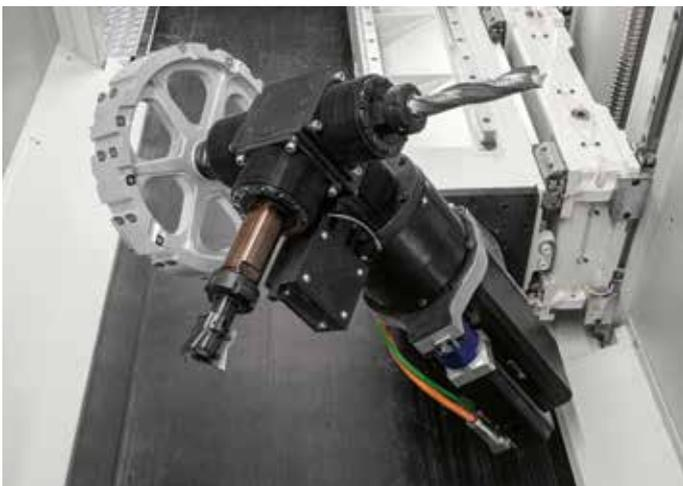
It is a device that is always ready for use as it is integral to the revolver unit and protected from dust thanks to a dedicated housing.
