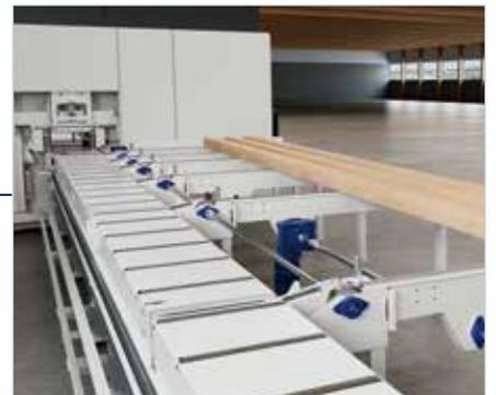
*Possibility of positioning a series of beams by means of the motorised chain loading system with buffer.*
