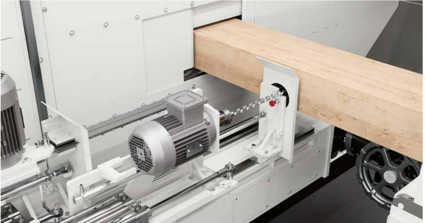
The horizontal drilling unit, positioned on the same crossbeam as the revolver unit, allows the execution of deep holes up to 450 mm from the workpiece front face. The operating unit includes a drill guide system in order to guarantee machining accuracy.
