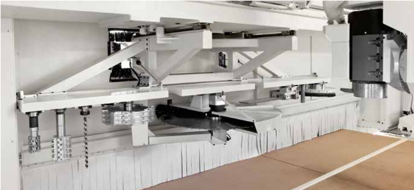
The tool store with up to 12 positions is designed to have on board all the tools necessary to complete the machining operations. Placed on the mobile gantry, it permits to have always available the right tool and to speed-up the execution time of the entire program.
